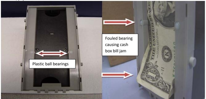
This can cause the bearings to not make full contact with the bill or completely stop it from moving. This condition will create bill jams, possibly leaving the bottom of bill slightly outside of the cash box. Dampen a lint free cloth with water (only enough water to pick up dust) and run the cloth up and down over the bearings until all debris is cleared.
