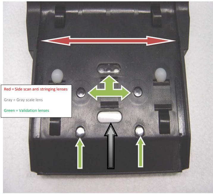
Inspect the plate for dust, dirt, smoke and debris. There are four round lenses and two oval lenses in the plate that must be cleaned. Dampen a lint free cloth with water, only enough water to pick up dust and run the cloth over all lenses and rollers until clean.
